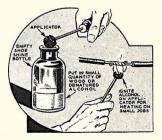
An empty shoe dressing buttle partly filled with denatured alcohol makes a practical torch for soldering splices in house wiring.
