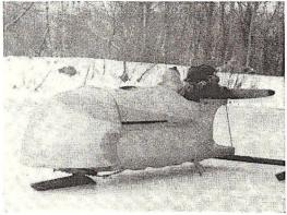
Powered by an old motorcycle engine and a small propeller, this snow-sled slides along at 62 m.p.h. Paul R. Bussler, Williamsport, Pa., built it from wood and sign painter's canvas.
