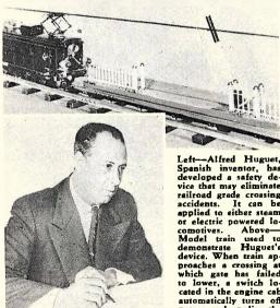
Spanish inventor, has developed a safety device that may eliminate railroad grade crossing accidents. It can be accidents. It can be applied to either steam or electric powered locomotives. Above-Model train used to demonstrate Huguet's device. When train apwhich gate has failed to lower, a switch lo-cated in the engine cab automatically turns off power and applies the brakes to train wheels.
