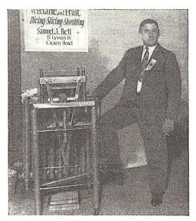
This machine will dice, slice, or shred any vegetable or fruit in one operation of the foot petal. A punch is set at the top and a die at the bottom. Each operation requires a die.
