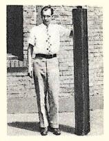
This 70-cell dry battery, 6 feet high, supplies power for one year. 85
