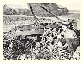
This beet farming machine slices tops off beets and digs them from ground 60 times faster than can be done by hand labor. John Devey, Jr.. of Glendale. Calif., invented the device.
