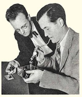
When the breath is blown through this apparatus iodine fume are given off and fingerprints immediately show up. Dr. John McMorris is shown demonstrating the device to an assistant.
