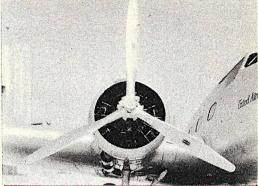
American airplanes equipped with Hamilton controllable pitch propellers like these above were instrumental in enabling Ekins to set a world's air travel record. They permit short takeoffs, maximum speed.
