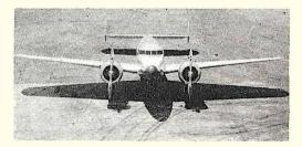
New twin-engine model transport which her buildets claim is America's fastest commercial plane. Built to carry six passengers and two pilots, its cruising speed is 213 m. p. h.
