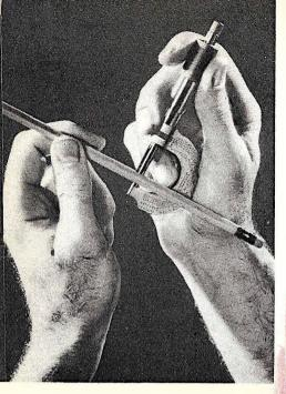
Within the thickness of the pencil in the calipers, 20,000 thin razor edges can be stacked. Each edge is one-eighty-thousandth of an inch.
